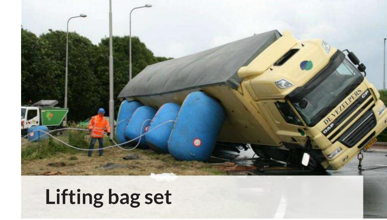
A complete set of Buitink Technology lifting bags comprises eight bags in **various different shapes and sizes**. A set has a total lifting capacity of no less than 68 tonnes!
