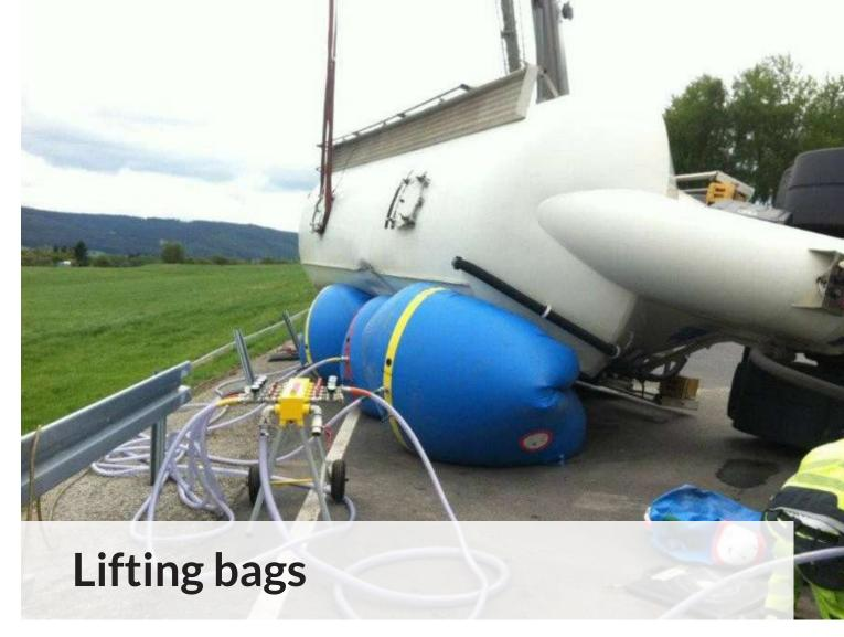
Buitink Technology develops and produces lifting systems for salvaging, among others, trucks with trailers, tipper trucks and coaches. The low pressure in the bags (approx. 0.5 bar/ 7.25 psi) and the large contact surface mean there is little risk of damaging an overturned truck.
