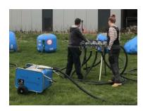
The air hoses provided are of an extremely high industrial quality, UV and weather resistant and also antistatic, so it's safe to work with flammable substances, for example, in the vicinity of the tanker trucks.
