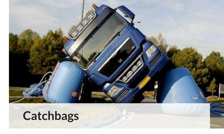
In addition to lifting bags, Buitink Technology also produces catch bags, or landing bags, for trucks. These ensure that trucks being salvaged with lifting bags end up nicely on their wheels after the tipping point.
